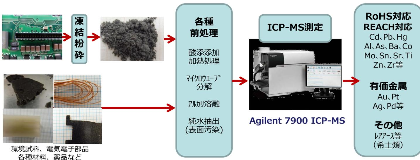
ICP-MS (Inductively Coupled Plasma Mass Spectrometry) : 誘導結合プラズマ質量分析計
