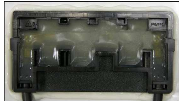
Filling state of resin in the terminal box (poly Si type)
